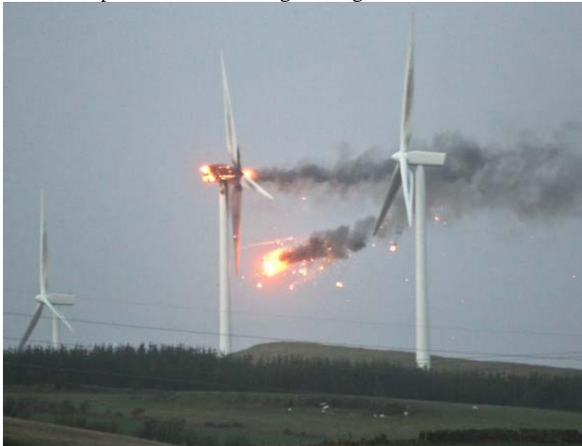
**Figure. 1.** Scottish windmill exploding in high winds on Dec. 8, 2011 (photo: Stuart McMahon)
