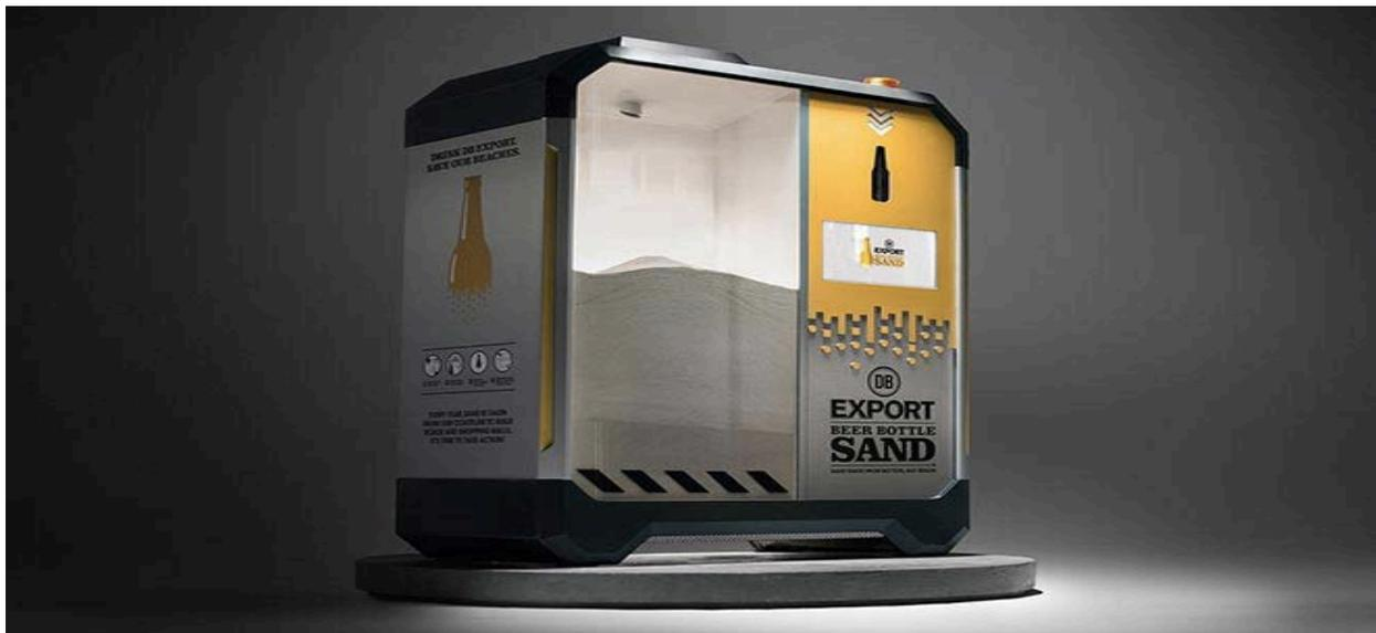
The Beer Bottle Sand Machines reduce an empty bottle of DB Export into sand substitute in just 5 seconds. As the bottle is inserted, a laser triggers a wheel of small steel hammers spinning at 2800 rpm. As the bottle is pulverized a vacuum
