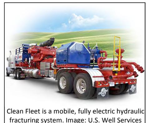
Clean Fleet is a mobile, fully electric hydraulic fracturing system. Image: U.S. Well Services
