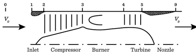
Figure 1, taken from Oates [3] shows a simplified cross section of an idealized fixed turbojet in an approaching ideal gas flow at flight velocity  $V_0$  and Mach number  $M_0$ . (The numbering of engine stations conforms to standard practice and the fuel mass addition is neglected.)
