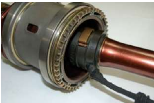
Sensor on Formula 1 half shaft
